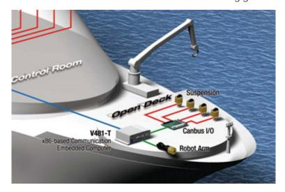
**Control Room:** The central control system connects other devices on the vessel and performs centralized management tasks. This is where you will find a wind sensor, time sync unit, and a computer that performs different tasks and communicates with the devices in the Open Deck and Bridge area. Additional devices include level gauges, alarms, loading calculators, and a UPS. With so many devices to manage, the embedded computer needs to support multiple CANbus and serial connectivity ports.
